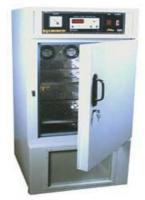
The heart of the our B.O.D. Incubator is the excellent and reliable solid state temperature controller cum indicator digital display, range from  $5^{\circ}$ C to  $60^{\circ}$ C  $\pm$   $0.5^{\circ}$ C.
